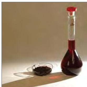
The synthetic blood paste solution in a dish (left) and with water added (right). (Photo provided by University of Sheffield)
